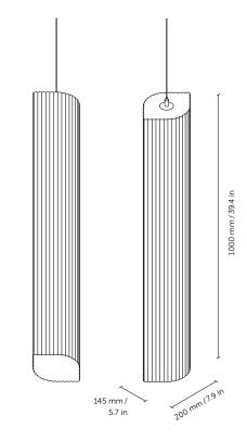
basic dimensions (w  $\times$  h  $\times$  d)  $200 \times 14000 \times 145$  mm  $/7.9 \times 39.4 \times 5.7$  in filling acoustic foam with high sound absorption surface finish flock (color refer to swatchers)
